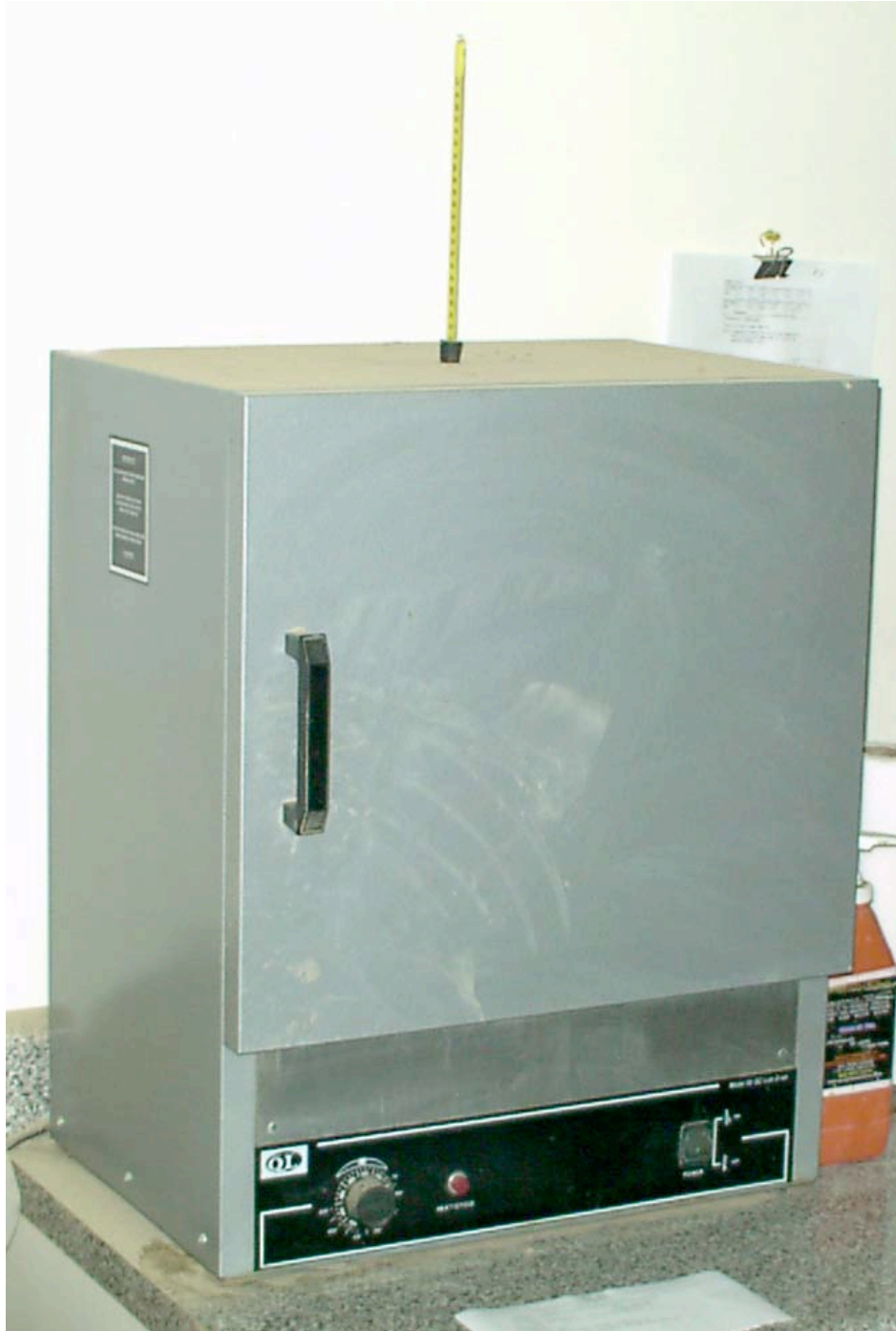
Figure 3-8 Drying Oven for Water Content Test
