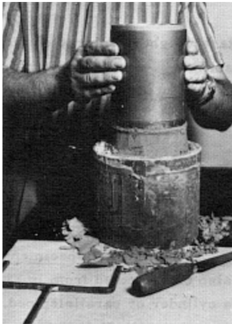
Figure 3-11 Determining the Unit Weight of a Soil Specimen with the Volumetric Cylinder (split-ring type)
