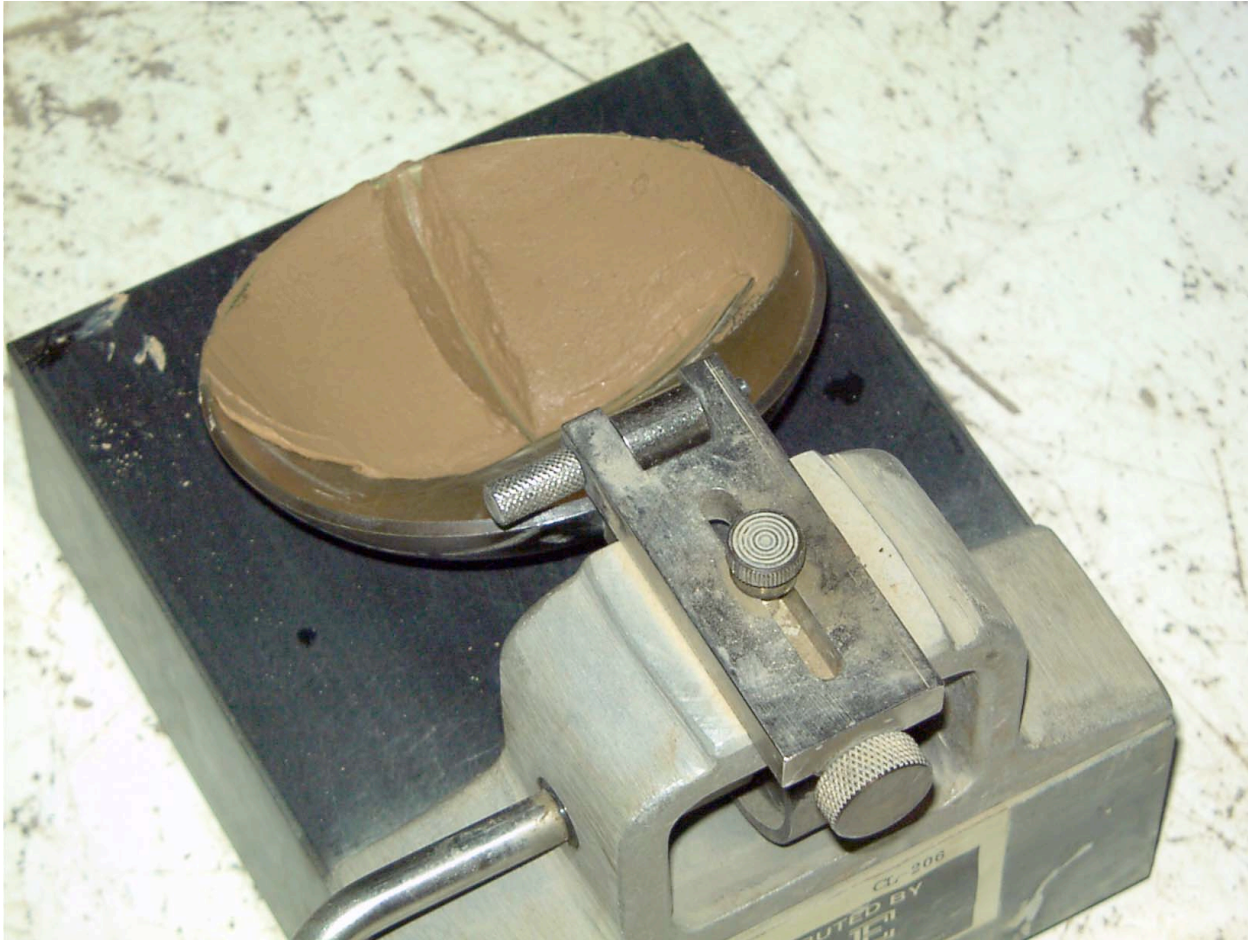
Figure 3-21 Soil pat after groove has closed
