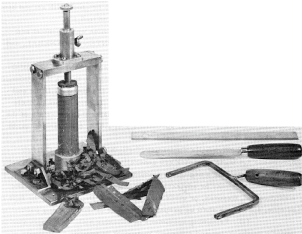
Figure 5-35 Squaring ends of specimen with a mitre box
