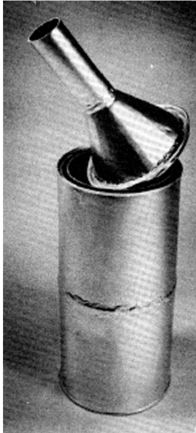
Figure 3-41 Pouring device, with 1" diameter spout
