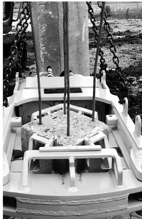
Feature (5). Crushers: for the Prime Concrete Pile Cutter. They are available in different shapes and sizes.
