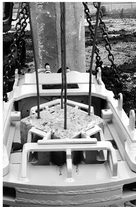
Feature (5). Crushers: for the Prime Concrete Pile Cutter. They are available in different shapes and sizes.
