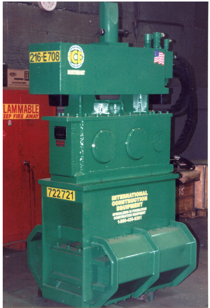
Figure 3-55 Excavator Mounted Vibratory Hammer with Wood Pile Clamp
