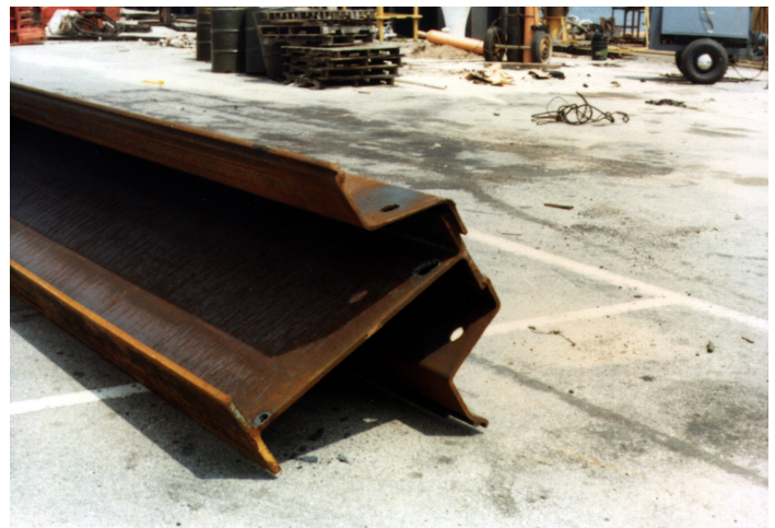
Figure 2-22 Master Pile Section
