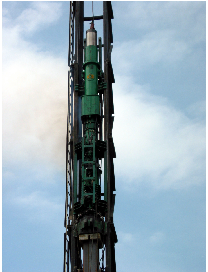
Figure 3-21 Open-End, Single-Acting Diesel Hammer
