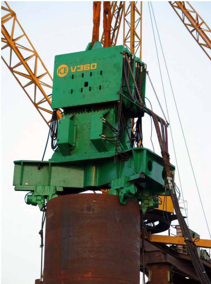
Figure 3-50 Caisson Clamp Arrangement for Large Caissons
