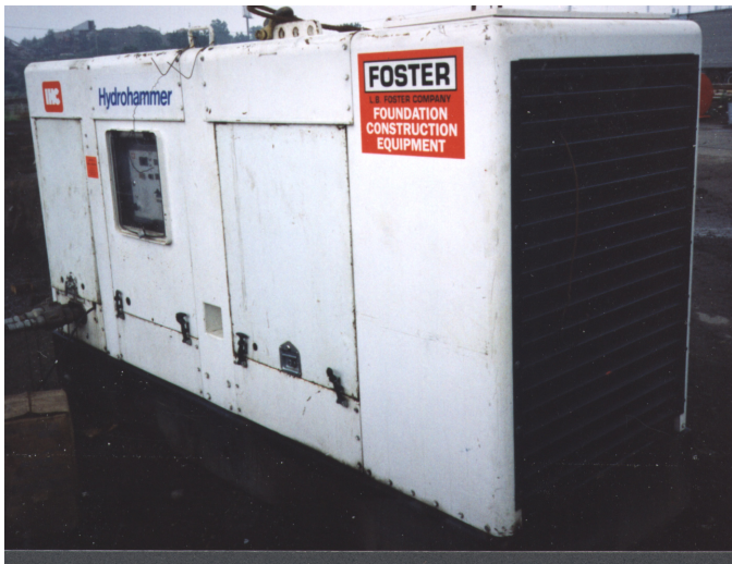
Figure 3-18 Hydraulic Power Pack
