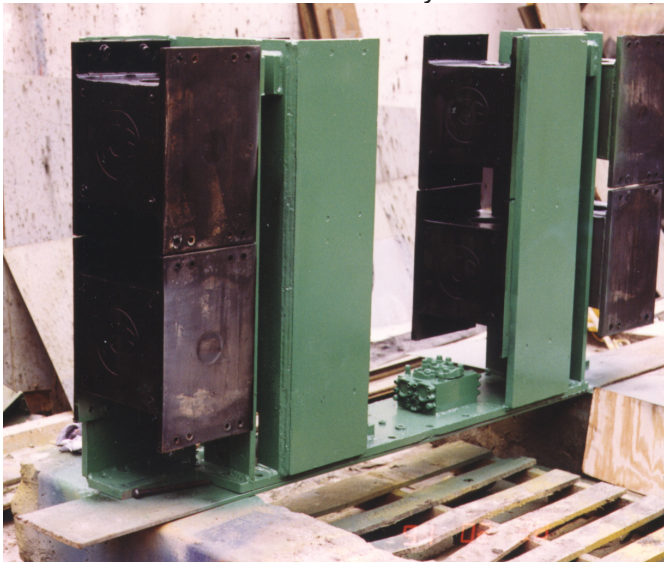
Figure 3-38 Elastomers or Springs Between the Vibrating and Non-Vibrating Portions of the Vibratory Hammer
