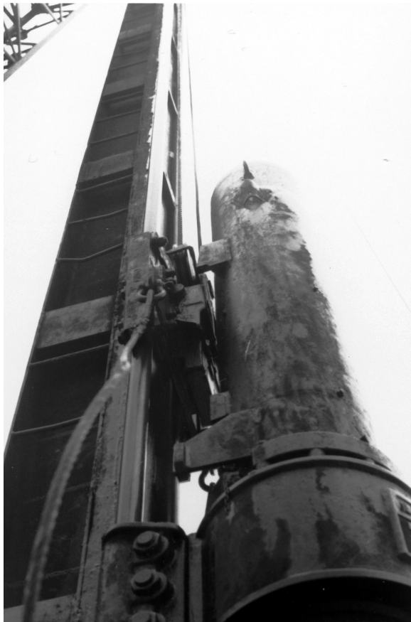
Figure 3-68 European or Spud Type Leaders with Hammer
