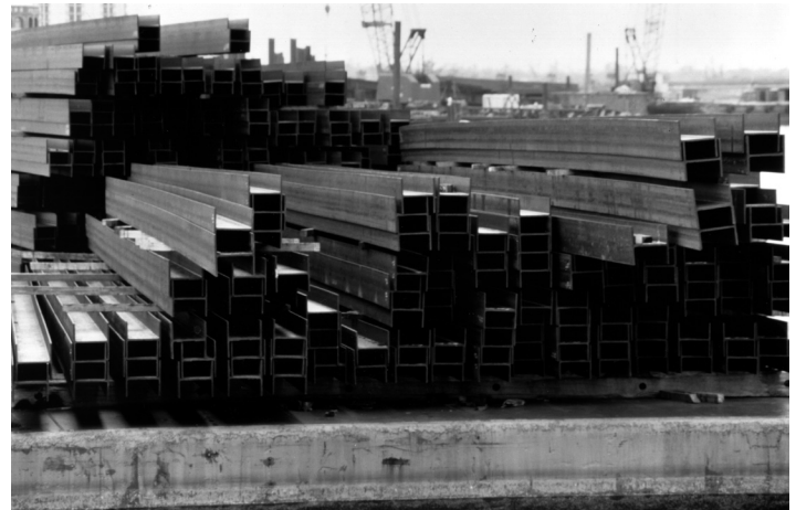
Figure 5-37 Proper Stacking of H-piles
