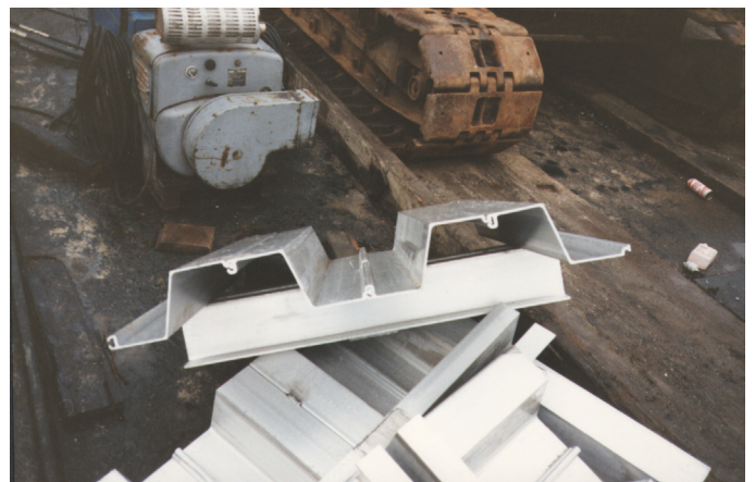
Figure 2-26 Aluminum “Z” Sections
