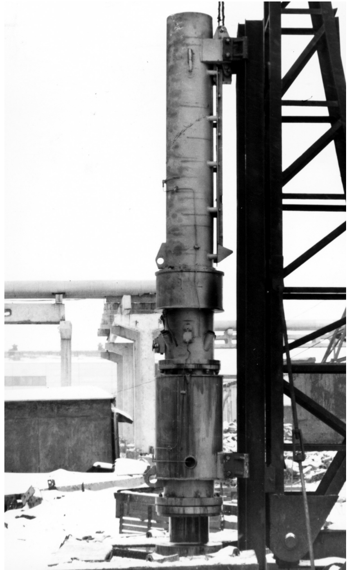
Figure 1-11 Water Cooled Diesel Hammer
