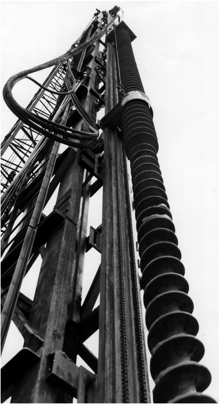
Figure 3-92 Auger Drill Assembly
