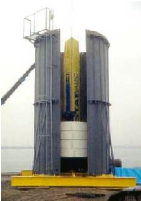
Figure 6-21 Statnamic™ Device with Canister for Gravel Catching and Reaction Weights
