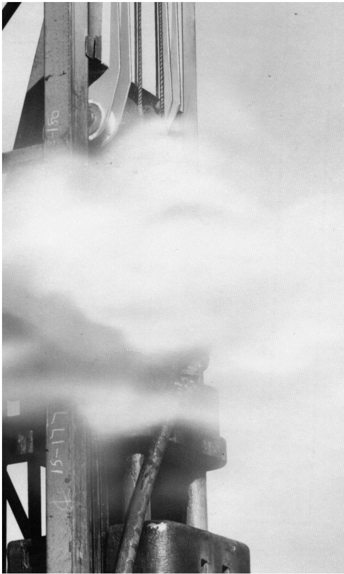
Figure 5-1 Exhaust Muffler for Air/Steam Hammers
